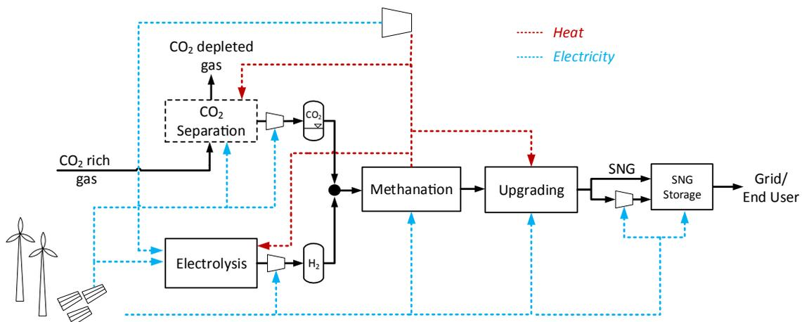
**Fig. 1.** Overview of a PtG plant with sub-system electrolysis for production of H<sub>2</sub>, sub-system methanation to convert H<sub>2</sub> and CO<sub>2</sub> into CH<sub>4</sub> and H<sub>2</sub>O. Before the gas is fed into the natural gas network or used for final purposes, it is upgraded and, if necessary, compressed. The dotted lines show the heat (red) and electricity flow (blue).
