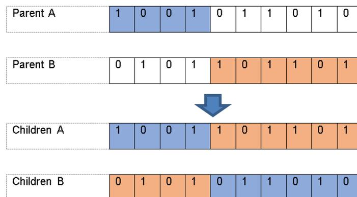
**Figure A-6-1:** Representation of the crossover operator
