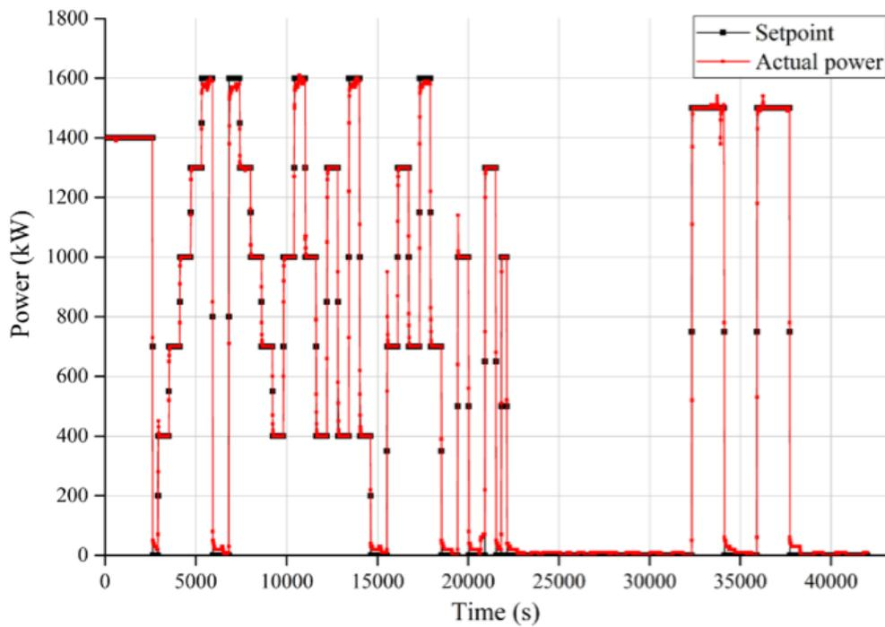
Figure 3-3 Falkenhagen test on an AEC-based electrolyser
