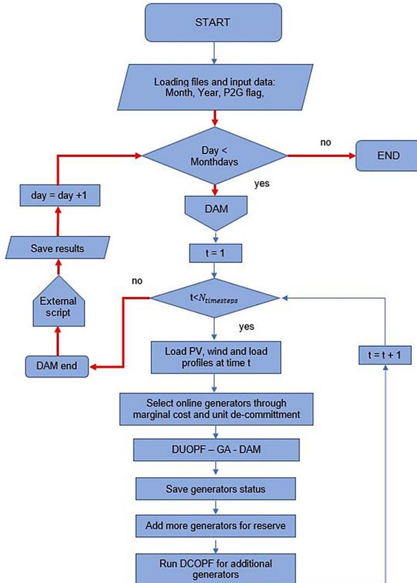
Figure B-6-2: Modified DAM flow chart
