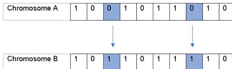
**Figure A-2:** Representation of Mutation operator
