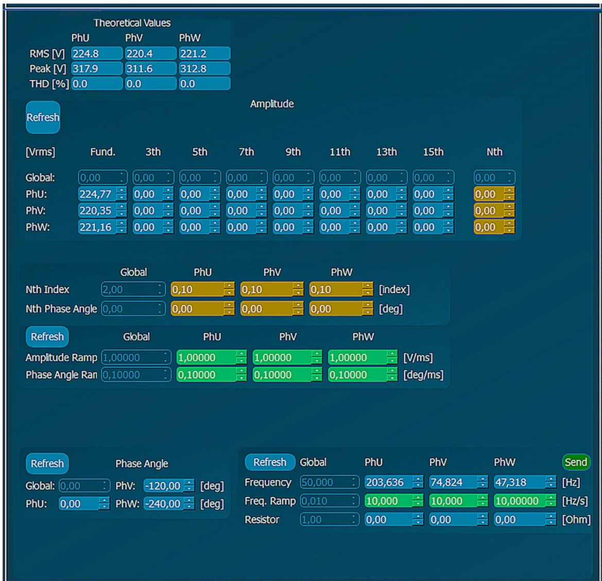
Figure 2-7: Cinergia’s AC configure panel
