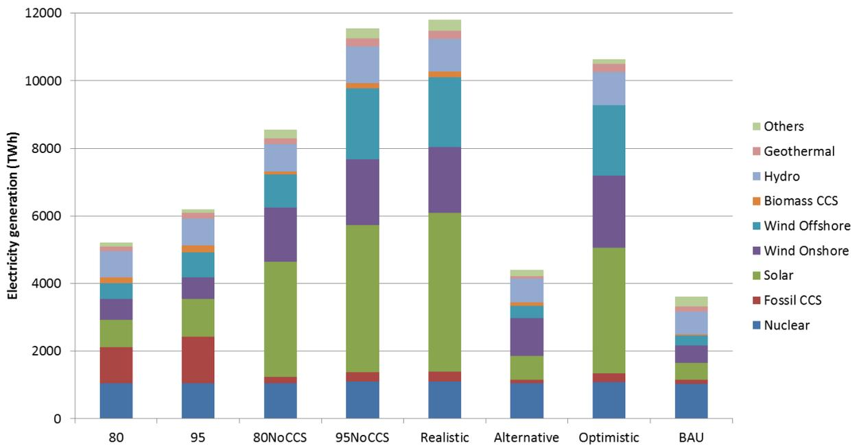
Figure 32. Technology contribution to electricity production in main scenarios.
