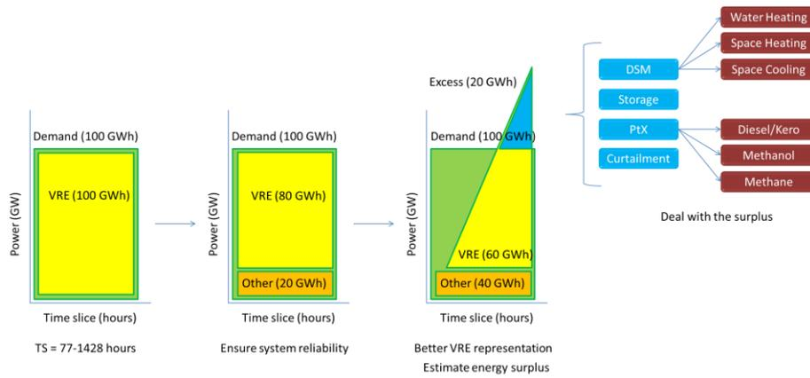
**Figure 29.** VRE representation and surplus estimation in JRC-EU-TIMES.
