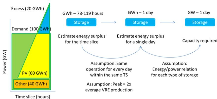
**Figure 30.** Storage sizing based on VRE surplus.
